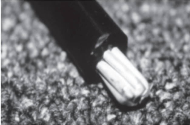
Figure H230-6 Covered conductor meeting Rule 230D
